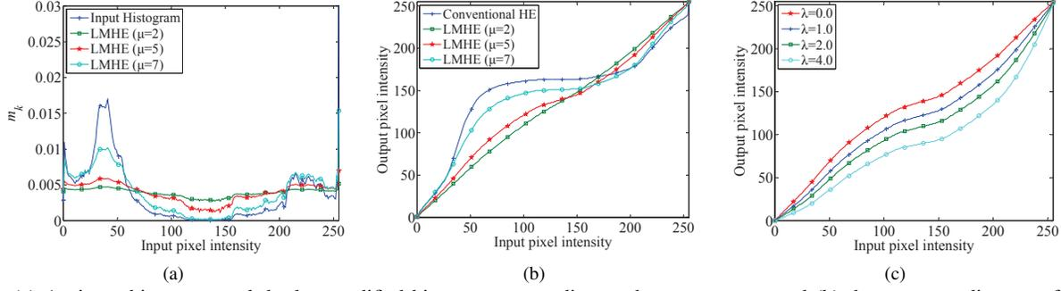
**Fig. 1.** (a) An input histogram and the log-modified histograms according to the parameter  $\mu$  and (b) the corresponding transformation functions when LMHE only is applied. (c) Power-constrained transformation functions for various  $\lambda$ 's when  $\mu = 5$ .
