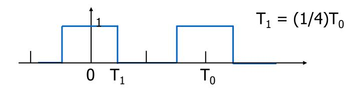
$$a_{k} = \frac{1}{T_{0}} \int_{T_{0}} x(t) e^{-jk\omega_{0}t} dt = \frac{1}{T_{0}} \int_{-T_{1}}^{+T_{1}} e^{-jk\omega_{0}t} dt$$
