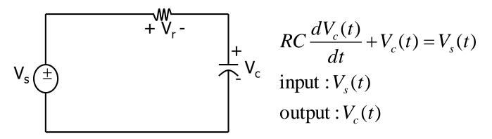
$$\therefore RC \frac{d}{dt} \Big[ H(j\omega)e^{j\omega t} \Big] + H(j\omega)e^{j\omega t} = e^{j\omega t}$$
