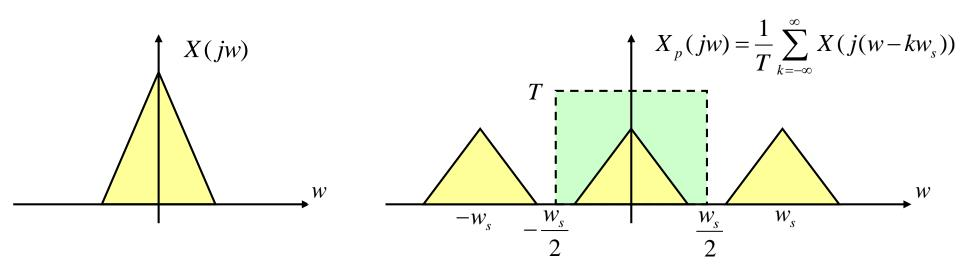
Reconstruction: ideal lowpass filter  $H(jw) = \begin{cases} T & |w| < \frac{w_s}{2} \\ 0 & \text{otherwise} \end{cases}$   $\Rightarrow h(t) = T \frac{\sin \frac{w_s}{2}t}{\pi t} = \frac{\sin \frac{\pi}{T}t}{\frac{\pi}{T}t} = \operatorname{sinc}(\frac{t}{T})$
