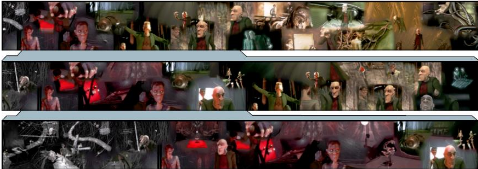
Figure 1: A multiscale tapestry represents an input video as a seamless and zoomable summary image which can be used to navigate through the video. This visualization eliminates hard borders between frames, providing spatial continuity and also continuous zooms to finer temporal resolutions. This figure depicts three discrete scale levels for the film Elephants Dream (Courtesy of the Blender Foundation). The lines between each scale level indicate the corresponding domains between scales. See the video to view the continuous zoom animation between the scales. For Copyright reasons, the print and electronic versions of this paper contain different imagery in Figures 1, 4, 6, and 7.
