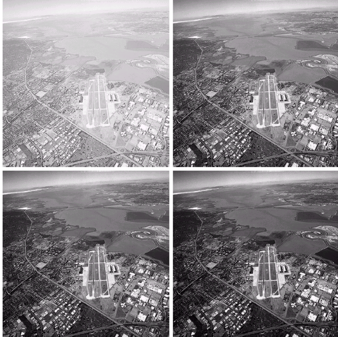
FIGURE 3.9 (a) Aerial image. (b)–(d) Results of applying the transformation in Eq. (3.2-3) with c = 1 and \gamma = 3.0, 4.0, and 5.0, respectively. (Original image for this example courtesy of NASA.)
