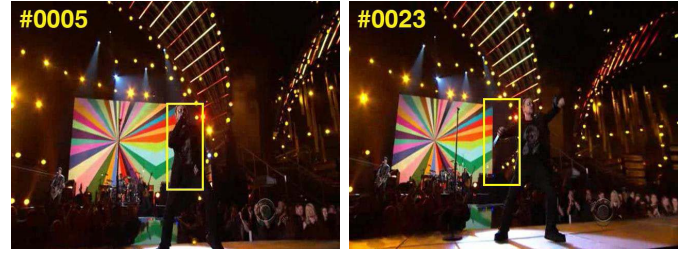
Fig. 3. Inclusion of background information within a bounding box due to a complex object shape. In this video, the background information causes a drift problem, causing the tracker to lose the target object eventually.
